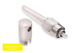
STRAN Technologies' High Reliability FC connectors have been designed for applications requiring excellent reliability in high shock, vibration, temperature and vacuum environments. All connector body parts are precission machined nickel plated brass. The FC's are available in a standard length and a short body version, ideal for tight spaces. The best choice for high reliability applications. Some of the applications supported by STRAN's High Reliability FC's and adapter include:
