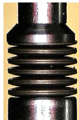
Figure 2. A stack of 11 Belleville washers comprise the M29504 spring.
